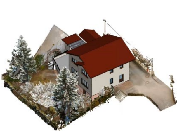
Overlay between point cloud and BIM model
